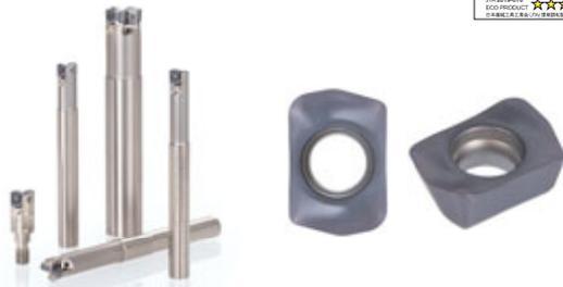
Low-resistance insert with thick corner and large-sized insert fastening screws that can withstand highly-efficient machining have been set. Positive inclination angle has improved chip treatment, which enables use in a wider application range as compared with conventional products.
