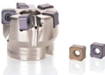
Face milling cutter designed to avoid tool interference. Even though the negative insert with double-sided specification is thick and has a strong cutting edge, it has low cutting resistance equivalent to a positive insert, which enables use in workpieces with thin wall/base or when the fixture is weak.
