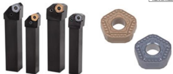
Economical with 10-cornered insert. Furthermore, adopting dovetail clamping for insert clamping has enabled stable highly-efficient machining. HD type holder with maximum 7-mm depth of cut and HF type holder with maximum 2-mm/rev feed are available, which enables use in a wider range of applications.
