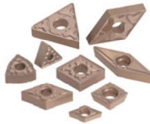
Al<sub>2</sub>O<sub>3</sub> layer with excellent heat resistance has been highly homogeneous structured and thickened by changing the material of the outer coating layer to high hardness ceramics. Furthermore, evolution of coating treatment technology to reduce defects in alloy base materials and to restrain progress of cracks gives this product excellent wear and fracture resistance.
