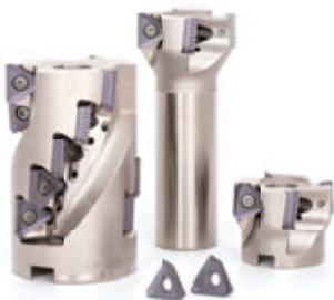
TungTriShred insert has two cutting edge varieties: serrated edges for roughing and straight lines for finishing. The unique pocket positioning ensures the cutting edge with a low cutting force and fewer gaps. TungTriShred provides high efficiency in roughing operation and good machining surfaces in finishing operation.
