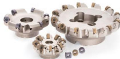
This face milling cutter has square, octagonal, and round inserts that can be fit in the same cutter body. The improved clamping structure reduces lifting of inserts and stress applied on the screws during heavy cutting.
