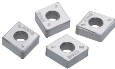
The brazing strength has been improved with the change of CBN brazing shape and the volume increase of CBN that has high thermal conductivity. Even in dry cutting, flaking on the CBN tip is unlikely to occur, and sudden fracture is prevented. The depth of cut can be increased by 1.6 times compared to the conventional product.
